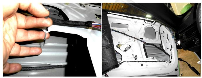
Now that you have gain the extra wire slack, cut the factory wire boot in half and pull the extra wire slack out as shown on the right.
