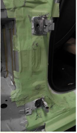
After grinding down the two-door hinge post place the new VDI hinge system against the two flat sections and mark the center of the holes. Try to get the holes as close to the center factory hinge post as possible. You will need to drill and tap one hole on at the
