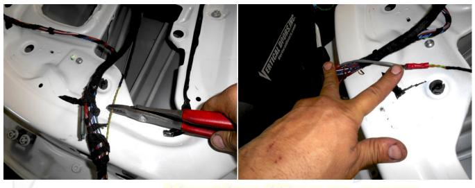
Make the wires to on a straight line and used "Zip ties" to secure the wires to the frame of the door.
