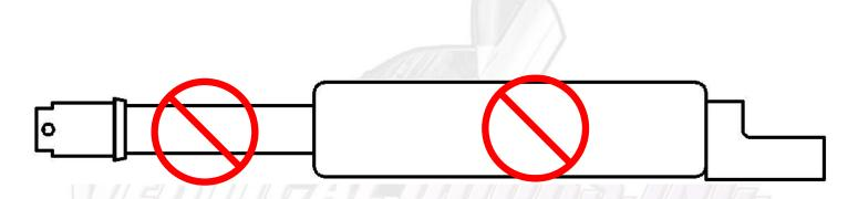
WARNING! THE USE OF ANY TYPE PLYERS, PAINT OR FOREING MATERIALS ON THE SHOCK'S BODY OR SHAFT WILL VOID THE WARRANTY.
