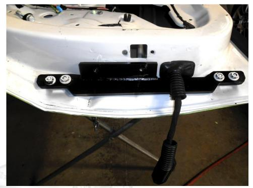
One the bracket is securely installed on the door now you can install the second section of the now VDI hinge system.
