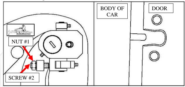
Hint\*(leave #1 nut loose until shock is installed Allen set screw will have to be re-adjusted after shock is installed.
